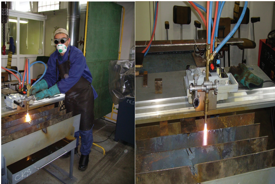
Fig. 3. Learning to cut steel with oxygen
