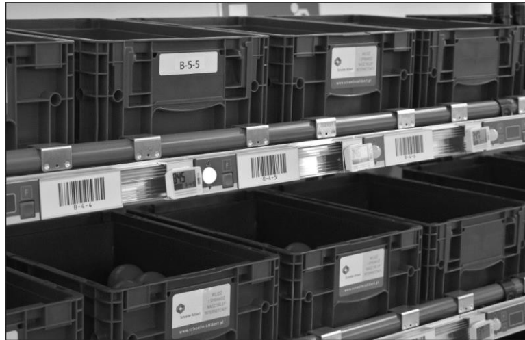
Figure 2. Shelf with the Pick-by-light system marked with a diode, the collection point of the assortment. Source: own study.
