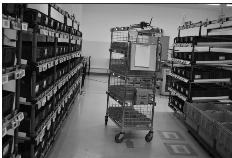
Figure 1. Pick-by-frame system trolley with visible pick-by-light diodes.
