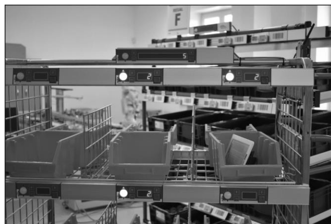
Figure 3. Pick-by-frame with a visible system of diodes, the numbers represent the quantity of goods that should be completed in the marked packaging. Source: own study.
